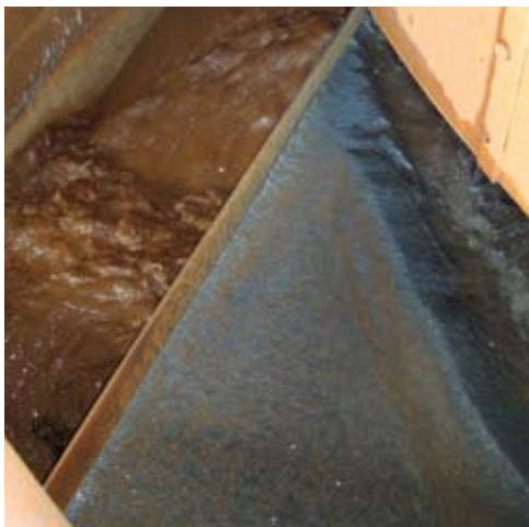
JONES rejects and concentrate of hematite ore in collecting launders
