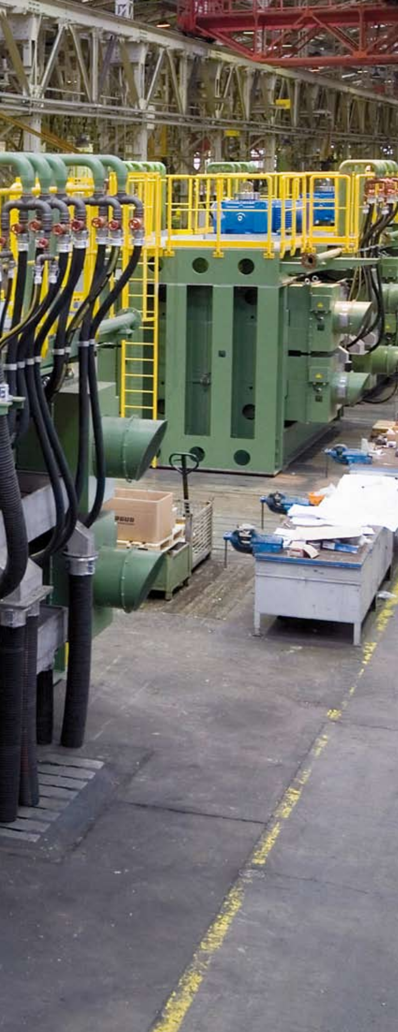
JONES WHIMS during no-load test run
