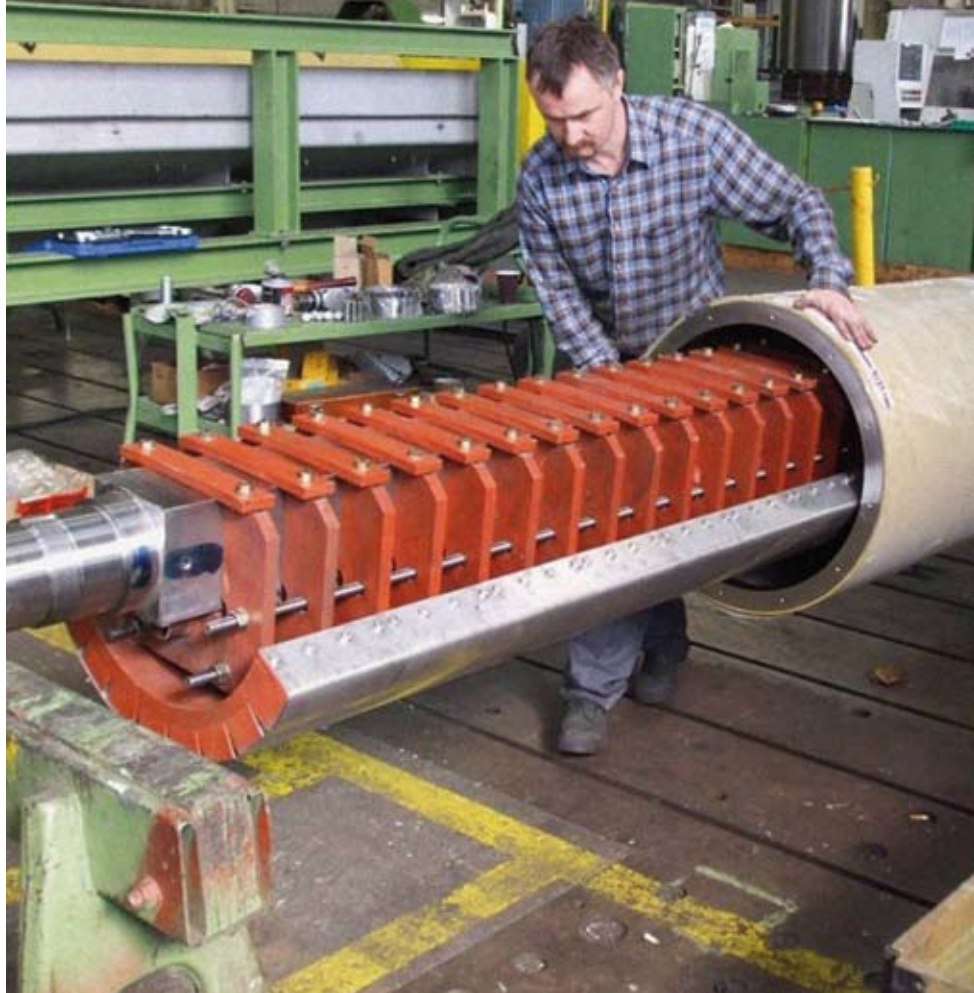
Installation of the magnetic system inside the drum
